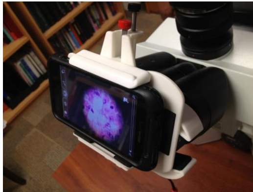
Figure 3. Cell phone adapter attached to a microscope supports telepathology
